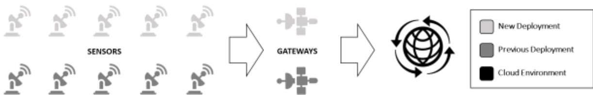
Figure 2. Physical architecture of the pilot
